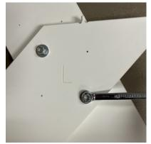
Finish this step by driving the two shorter screws into the pre-drilled holes.
