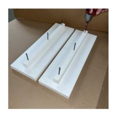
Using pre-drilled holes, fasten one stiffener per seat board with screws. Make sure the rounded corners are facing out. (If installing Bench as opposed to Chair – 8 screws will be used).
