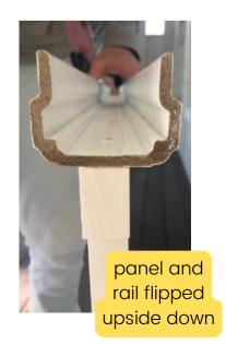
Make sure the PVC Panel rests in the middle of the bottom outer rail, and screw through rail into panel using 1-5/8" exterior deck screws (not provided). Be sure to screw every 6" as well as on either side of seam where panels are joining.
