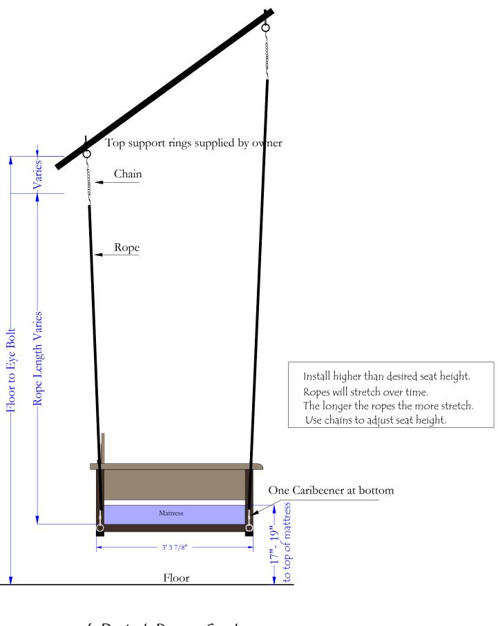
4 Point Rope System Sloped Ceiling
